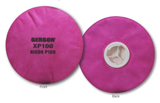
**NIOSH Approved** P100 filter for use with Gerson Half Masks and Full Face Respirators. At least 99.97% filtration efficiency against solid and liquid aerosols, including oil-based aerosols.
